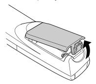
2. Insert the two AA batteries included with the projector. Make sure the polarity of the batteries is correct.
