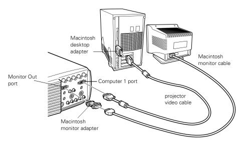
1. Connect one end of the projector video cable to the projector's Computer 1 port. (Use the Computer 2 port if you are connecting a second computer.)
