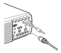
2. To use the remote control as a wireless mouse, connect the PS/2 or USB cable included with the projector to the MOUSE terminal on the square end of the main cable.
