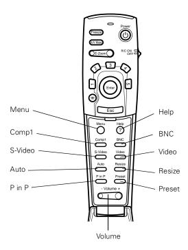
The remote control uses a line-of-sight infrared signal. To use the remote control, point it toward one of the remote control receivers located at the front and back of the projector. (See page 62.)
