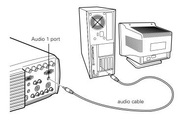
2. Connect the other end of the audio cable to the speaker or audio out port on the computer's sound card.
