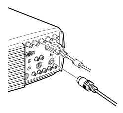
2. To use the remote control as a wireless mouse, connect one end of the projector's Mac mouse or USB cable to the MOUSE terminal on the large end of the main cable.
