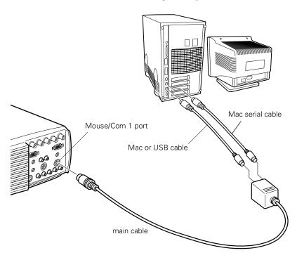
1. Connect the small end of the main cable to the projector's Mouse/Com 1 port. (Use the Mouse/Com 2 port to connect a second computer.)
