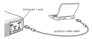
1. Connect one end of the projector video cable to the projector's Computer 1 port. (Use the Computer 2 port if you are connecting a second computer.)
