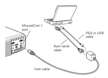
Connect the round end of the main cable to the projector's Mouse/Com 1 port. (Use the Mouse/Com 2 port if you are connecting a second computer.)
