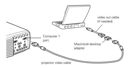
**Note:** Some new PowerBooks may allow you to connect the video cable directly to the computer without using a video-out cable. See your PowerBook manual for additional information on connecting a video cable.
