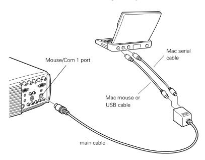
1. Connect the round end of the main cable to the projector's Mouse/Com 1 port. (Use the Mouse/Com 2 port if you are connecting a second computer.)
