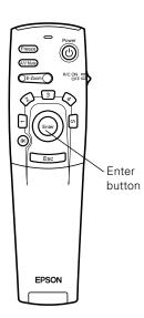
3. Press the Enter button to display a submenu.
