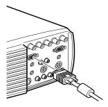
2. Connect one end of the projector video cable to the projector's Computer 1 port. (Use the Computer 2 port if you are connecting a second computer.)
